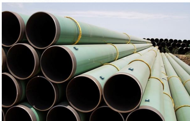
Figure 2. An RFID tagged pipe joint is easily found.
